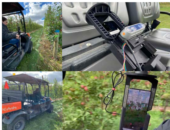
Figure 1. Scanning of an orchard using Farm Vision equipment, including cellphone, RTK GPS, and battery pack, affixed to stabilizing device (3 ft pole). This equipment will no longer be used in 2023. Harvest scans were conducted with two people using an ATV. One person drove the ATV and a cell phone operator scanned full rows (both sides) as shown in the cell phone screen. Photo: Mario Miranda Sazo.
