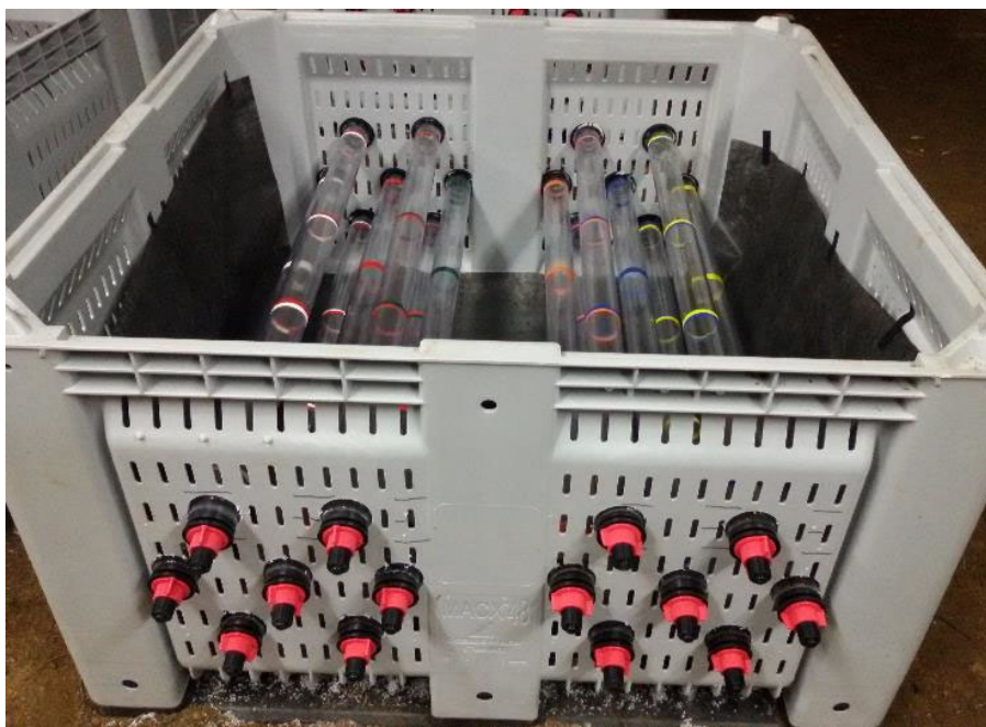
Figure 3. Tube rhizotron systems to study rootstock interactions with soil pH.
